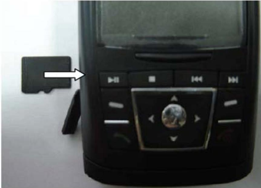
Install the memory card: find the location of the memory card slot, push the card in direction of the arrow, and push it until it reaches the lock position. When installing a memory card, please confirm that the metal contacts of the card is downward (shown as the figure).
