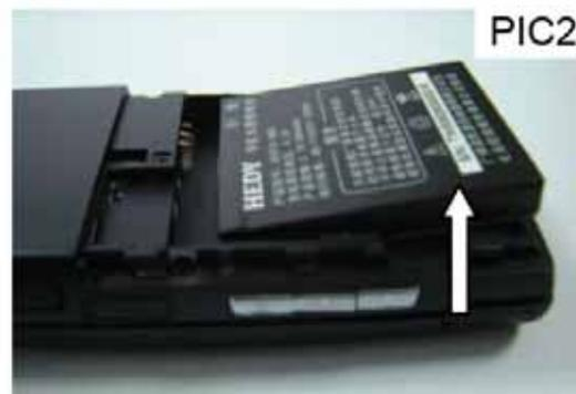
Install: ①Insert the battery;②Push the battery cover until you hear “kaka”
